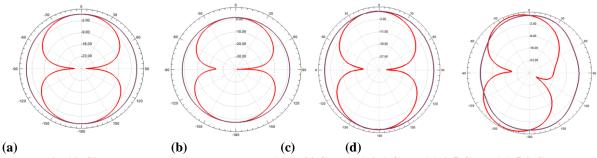
Fig.12. Simulated Radiation Patterns at (a) 2.44 GHz, (b) 3.1 GHz, (c) 3.5 GHz, (d) 5.2 GHz
