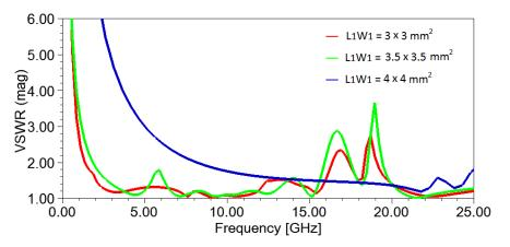
Fig.6 VSWR plots for the variation in the slot L<sub>1</sub>W<sub>1</sub>
