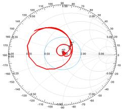
Fig.13. Simulated Smith chart of Dual-band Antenna
