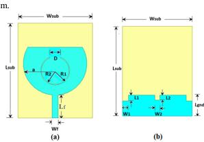
Fig.1. Design of the proposed modified circular-shaped printed monopole antenna with the circular arc slot.
