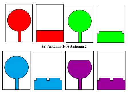
(c) Antenna 3(d) Antenna 4 Fig.2. Development of modified circular-shaped UWB monopole antenna.
